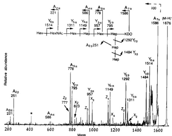
FIG. 3. MS/MS spectrum of underivatized oligosaccharide from *H. ducreyi* strain 35000. The peak at  $m/z$  413 which is marked by an asterisk is unassigned. KDO is anhydro-KDO.
