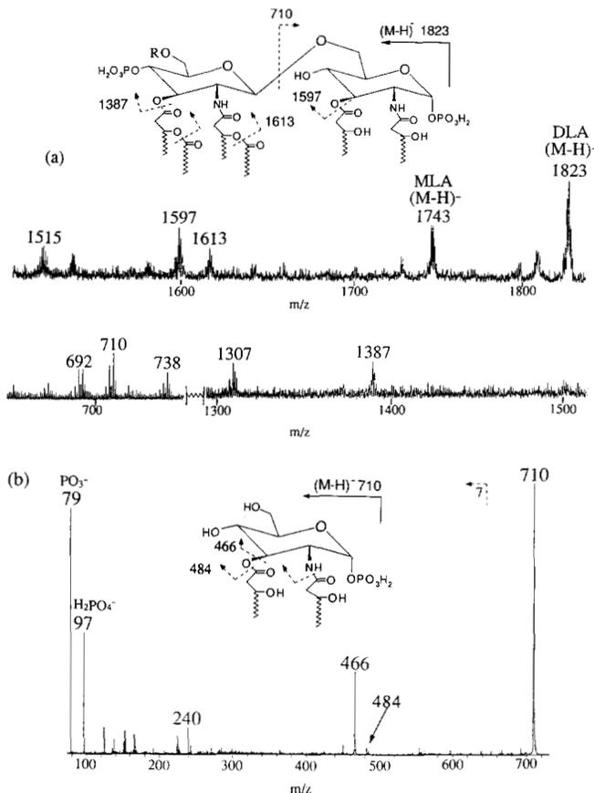
FIG. 5. *a*, LSIMS spectrum of the lipid A from *H. ducreyi* strain 35000 and *b*, the corresponding MS/MS spectrum of one of the major fragment ions at  $m/z$  710.
