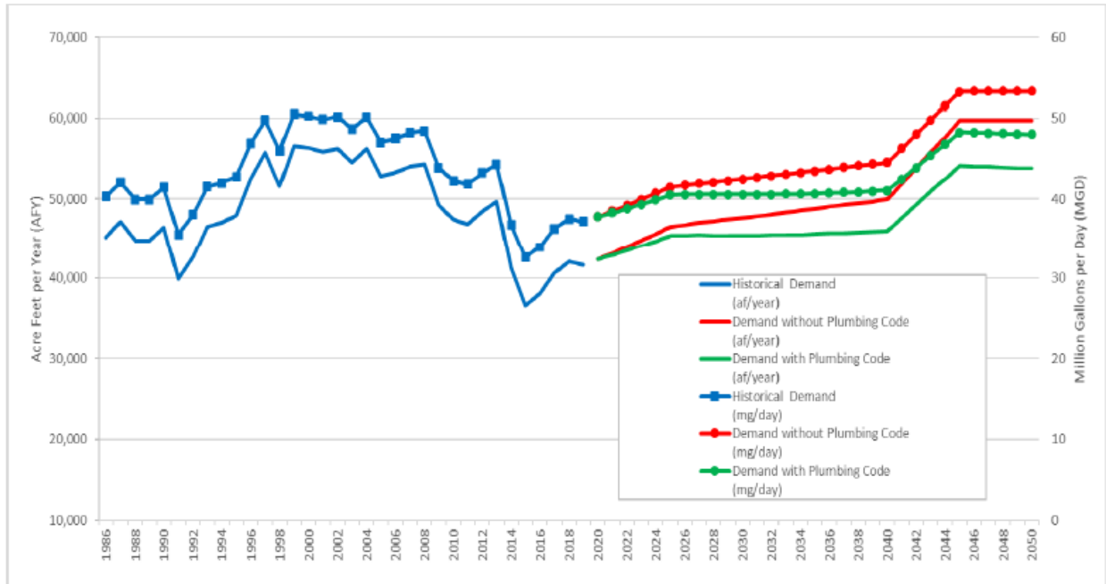
Figure 4: Alameda County Water District’s projected water demand with plumbing code savings. The blue solid line shows historic water demand in acre-feet per year, while the dashed line shows the same but in million gallons per day. The red solid line shows the projected demand if plumbing code efficiencies were not mandated in acre-feet per year, while the dashed red line shows the same but in million gallons per day. The green solid line shows the projected demand if plumbing code efficiencies were mandated in acre-feet per year, while the dashed green line shows the same but in million gallons per day (ACWD b , 2021).
