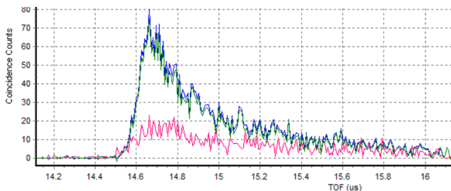
Figure 3.3.2b: An asymmetric TOF peak is detected in 0 K ethylenediamine photodissociation at 9.125 eV using TPEPICO. Data taken at University of the Pacific on May 31, 2015. The signal from the center detector is blue, the signal from the ring detector is red, and the corrected center signal using a factor of 0.22 is shown in green. These non-Gaussian peak shapes are representative of slow dissociation reactions.
