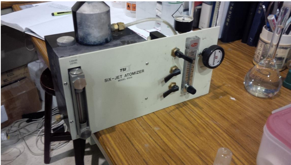
Figure 3.2.3a: The six-jet TSI Inc. Model 9306 atomizer used in the photoelectron spectroscopic studies at the NSRRC.
