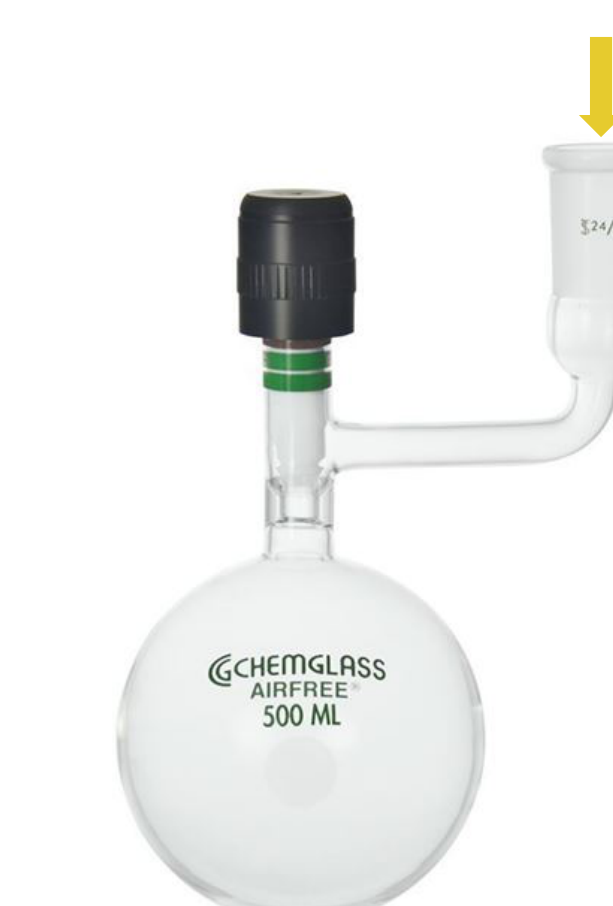
Figure 8. Material added through side arm of bomb flask. (CHEMGLASS, 2020)
