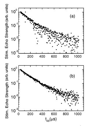
FIG. 6. Stimulated-photon-echo decay on the  ${}^4I_{15/2}(1) \rightarrow {}^4I_{13/2}(1)$  transition in  ${\rm Er}^{3+}$ : Y<sub>2</sub>SiO<sub>5</sub>. Each point represents a single shot. (a) Measured with a free-running laser. (b) Measured with a laser stabilized to a spectral hole and inhomogeneous line at field B=0.2 T.
