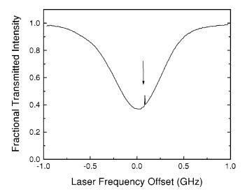
FIG. 1. Transmission spectrum of 0.005% Er<sup>3+</sup>:Y<sub>2</sub>SiO<sub>5</sub> scanned by a diode laser showing the entire inhomogeneously broadened absorption profile at zero applied field (B=0 T). The arrow indicates a spectral hole burned by a second laser.
