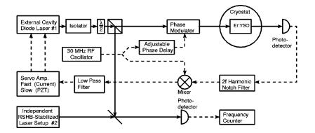
FIG. 2. Experimental apparatus for laser frequency locking to spectral holes and beat frequency measurement of laser stability (by combining the beam from the laser shown and that from an independent second laser system).
