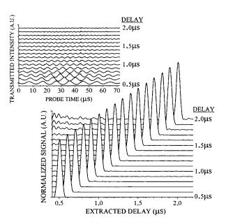
FIG. 2. Normalized traces of extracted time delay data are shown for processed time delay  $\tau_D$  values ranging from 0.5–2.0  $\mu$ s, after 800 shots using a 25 mW processing beam. The inset shows traces of the frequency-swept probe, which map the corresponding accumulated spectral gratings.
