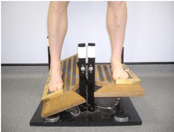
Figure 1: Tilt platform simulating a nonpathological lateral ankle sprain used for muscle reaction time testing.
